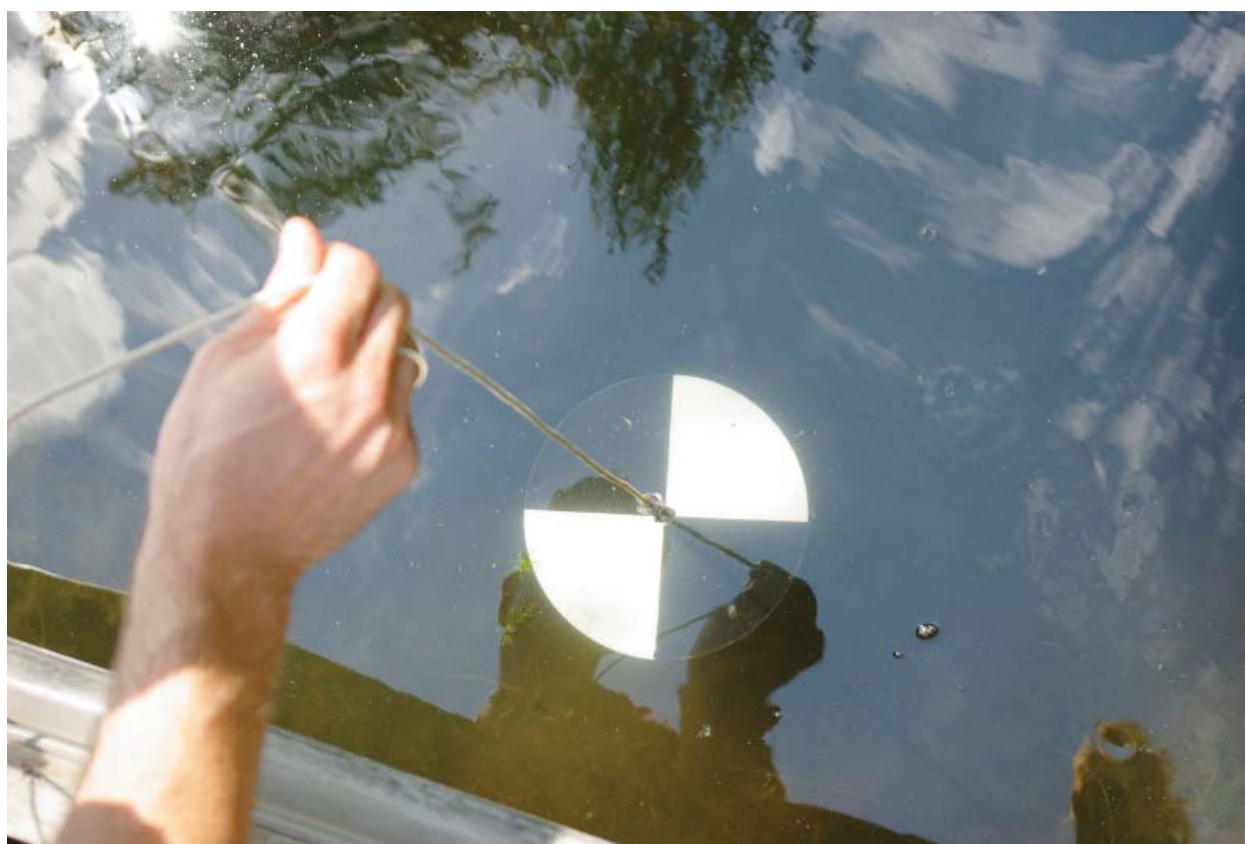
Figure 3 Measuring Water Clarity with a Secchi Disk
